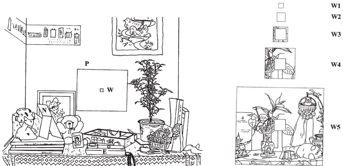
Figure 1. Front view in the subject room (left) and view of the test room under different size of windows (right) [3].
