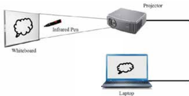
Figure 1: Basic Framework of Interactive Projection System Overview
