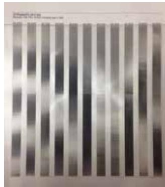
Figure 4 the first test chart for defining the correlation of the resolution of the lens and the printer
