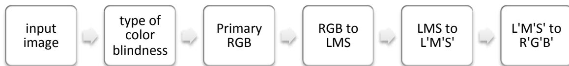
Figure 3. Method of colour converting for creating colour blindness simulation (6)
