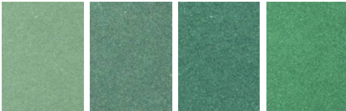
Fig. 1: Photographs of panels made of green interference pigments with rising saturation: Iriodin ® 9231, Iriodin ® 9235, Iriodin ® 97235 and Pyrisma ® T40-24 SW Green (from left to right)
