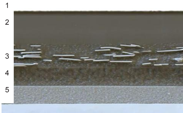
(1)air, (2)clear coat, (3)base coat (15 \mu\text{m} thick), (4)filler layers and (5)substrate
